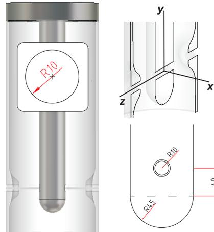
Figure 2: The nominal high- $\beta$  cavity (left), the co-ordinate system (top right) and the geometry of the internal conductor (bottom right). Dimensions in mm.
