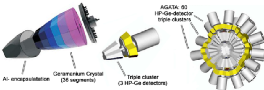
Figure 3.4: The AGATA HPGe detectors [2].
