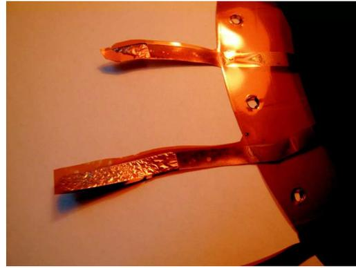
**Figure 6.** Polymeric deposits on the electrode.
