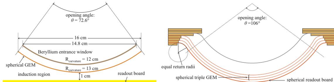
**Figure 3.** Schematic composition of two prototypes based on spherical GEMs. Left: single spherical GEM with spherical drift electrode but flat readout structure. Right: an entirely spherical triple GEM detector
