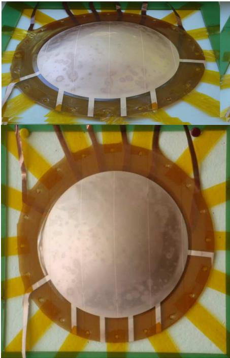
**Figure 7.** Spherical GEM made in a vacuum of  $\sim 10$  mbar.
