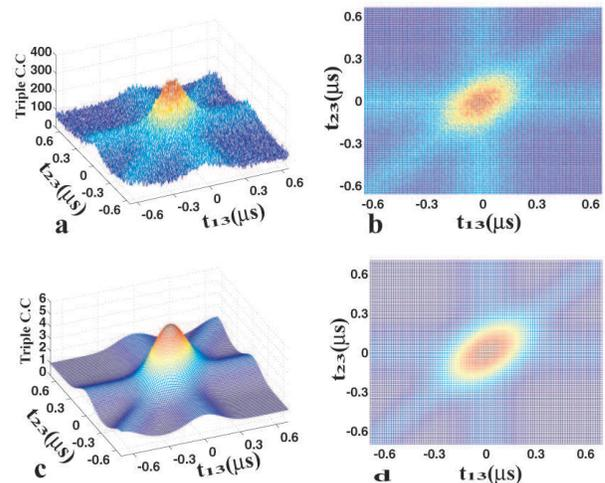
FIG. 2: (Color Online) Measured (upper, a and b) and calculated (lower, c and d) third-order temporal correlation joint function of thermal light. The 3-D three-photon joint detection histogram is plotted as a function of  $t_{13} \equiv t_1 - t_3$  and  $t_{23} \equiv t_2 - t_3$ . The simulation function is calculated from Eq. (5). In addition, the single detector counting rates for  $D_1$ ,  $D_2$ , and  $D_3$  are all monitored to be constants.
