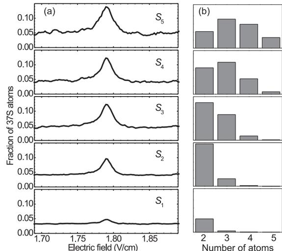
FIG. 1: (a) Experimental spectra  $S_1 - S_5$  of the Förster resonance  $\text{Rb}(37P_{3/2}) + \text{Rb}(37P_{3/2}) \rightarrow \text{Rb}(37S_{1/2}) + \text{Rb}(38S_{1/2})$  for 1–5 detected Rydberg atoms. (b) Theoretical probability distributions given by Eqs. (2) and (3) for the number of actually interacting Rydberg atoms.
