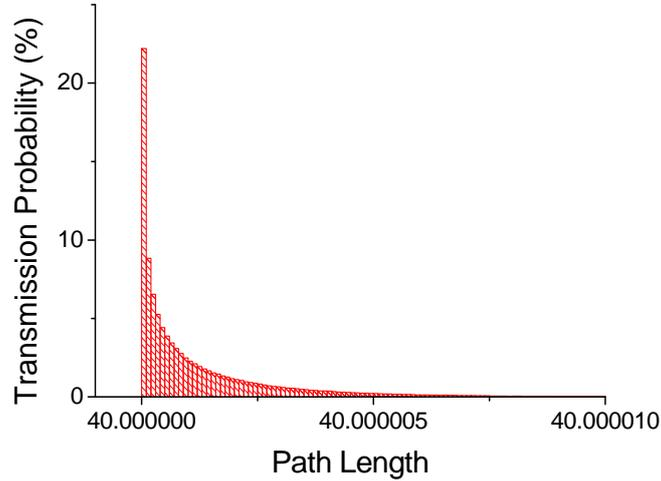
Fig.2. Numerical simulations of Fig. 1. For Eq. (1), path length is  $\ell = 40$ :  $L=2$ ,  $d=0.1$ , and  $n=1$ . The path length is obtained by using 1,000,000 rays for  $L/d = 20$ . The input pulse forms a Gaussian profile in the middle of the notch  $d$ . The beam size and the maximum divergence are  $0.2d$  and 1 milliradian, respectively.
