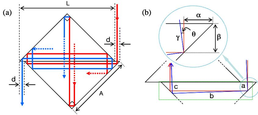
Fig. 1. Schematic of optical delay system using a prism pair for (a) vertical incidence and for (b) path difference diagram between vertical and angled incidence.
