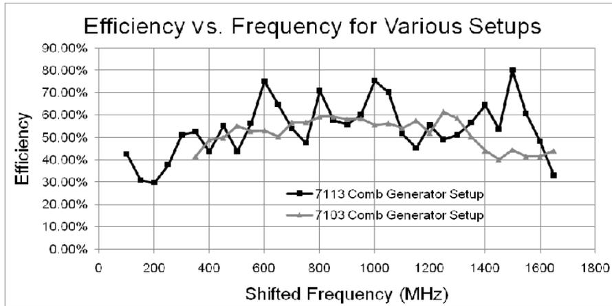
Fig. 3. Performance of the two NLTLs when the input waveform is optimized for each frequency as described in the text
