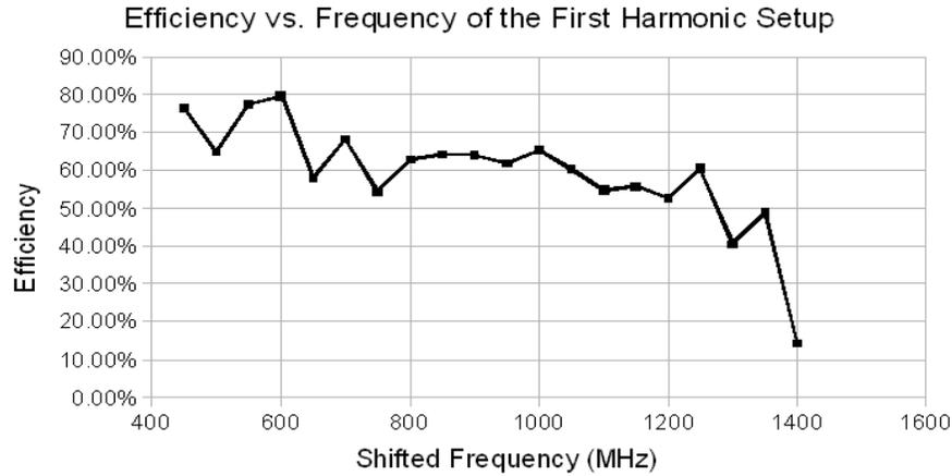
Fig. 5. Graph of the performance of the 7103 comb generator with first harmonic mixed into the input
