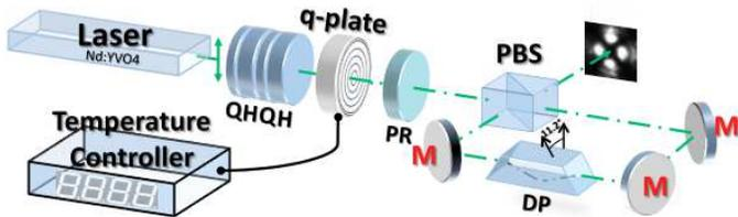
FIG. 1. (Color online) Experimental setup for generating polarization-controlled linear combinations of  $LG_2$  beams. Legend: QHQH - set of waveplates to control the beam polarization; PR - polarization rotator; PBS - polarizing beam splitter; DP - Dove prism; M - mirror.
