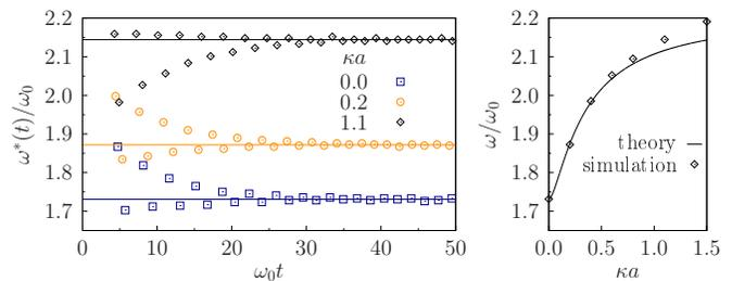
FIG. 2: (Color online) Left: Instantaneous oscillation frequency of  $E_{\text{pot}}$  (cf. Fig. 1) for various  $\kappa$  at  $\nu/\omega_0 = 0.1$ . Horizontal lines denote the mean frequency in the interval  $35 \leq \omega_0 t \leq 50$ . Right: Mean frequency (corrected for friction, see text) compared to the analytical expression of Ref. [21].
