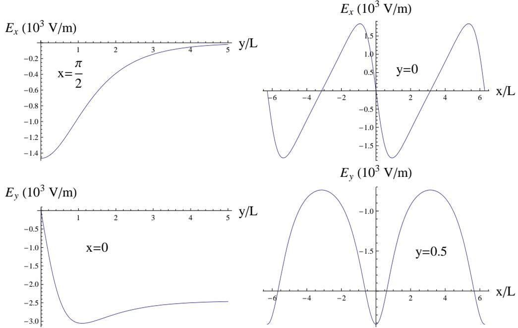
Figure 2: Profiles of the electric field components  $E_x$  and  $E_y$  associated with the cat-eyes solution (7). The profiles  $E_x(y)$  and  $E_y(x)$  have chosen at  $x/L = \pi/2$  and  $y/L = 0.5$ , respectively, because  $E_x(x = 0, y) = E_y(x, y = 0) \equiv 0$ .
