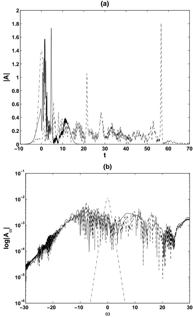
FIGURE 1. Spectral (bottom) and temporal (top) picture of the pulse profile at  $z = 0$  (dash-dotted),  $z = 10$  (solid) and at  $z = 100$  (dashed). Parameter values  $\epsilon = 0.01, c_2 = 0.001, c_3 = 0.01$ .
