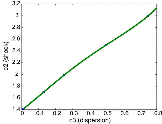
FIGURE 7.  $c_2$  vs  $c_3$  curve that separates regions where the numerical simulation blows up (region above the curve) from the region where supercontinuum is numerically observed (region below the curve).
