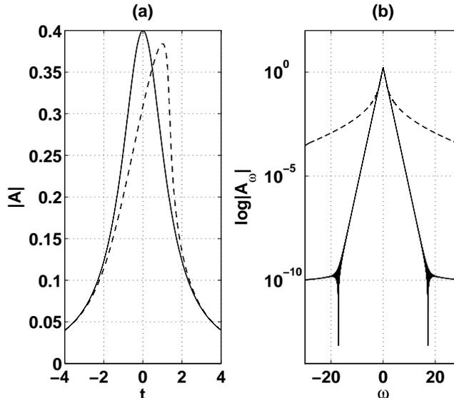
FIGURE 8. (a) The initial pulse (solid) and output pulse (dashed) after propagation  $z = 5$ , resulted from Eq.(14), where  $\chi^{(1)} = 0$  and  $\chi^{(3)} = 1$ . (b) Spectra of initial pulse (solid) and output pulses (dashed).
