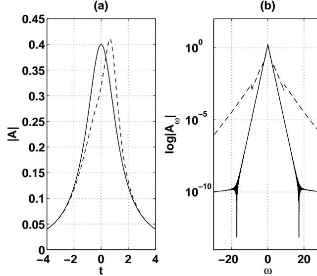
FIGURE 10. (a) The initial pulse (solid) and output pulse (dashed) after propagation  $z = 5$  with combining linear and nonlinear effects. The solution is computed based on Eq. (14), where  $\chi^{(3)} = 1$  and  $\chi^{(1)}$  as in Eq. (15). (b) Spectra of initial pulse (solid) and output pulse (dashed) presented.
