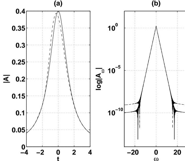
FIGURE 9. (a) The initial pulse (solid) and output pulse (dashed) after propagation  $z = 5$ , resulted from Eq.(14), where  $\chi^{(3)} = 0$  and  $\chi^{(1)}$  as in Eq. (15). (b) Spectra of initial pulse (solid) and output pulse (dashed).
