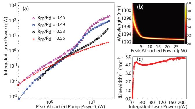
FIG. 4: (a) L-L curves of several devices of increasing  $R_m/R_d$ . (b) Normalized spectra versus pump power and (c) inverse linewidth versus output laser power for a device with  $R_m/R_d = 0.42$ .
