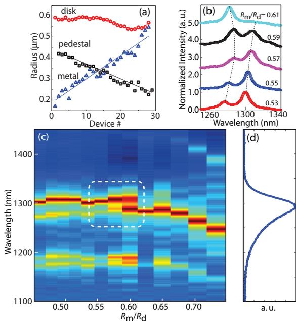
FIG. 3: (a) Measured disk, metal, and pedestal radii of fabricated device array. (b) Zoom-in of anti-crossing region as indicated by a dashed white box in panel (c). Dotted lines are guides to the eye. (c) Fiber-taper-collected normalized spectra on a log-scale as a function of  $R_m/R_d$  ( $P_p = 1$  mW,  $\delta T = 500$  ns,  $T = 1$   $\mu$ s). (d) Free-space-collected PL of un-patterned laser material ( $P_p = 282$   $\mu$ W, continuous-wave).
