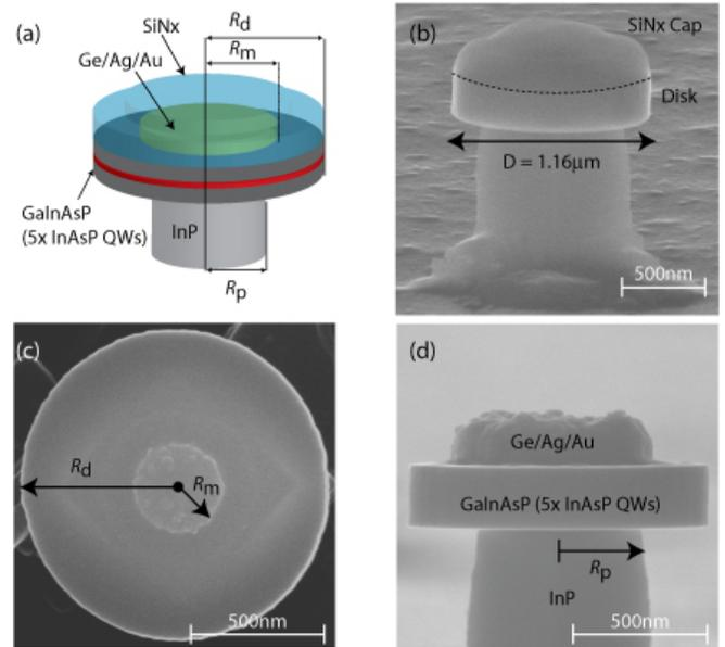
FIG. 1: (a) Schematic of fabricated and simulated microdisks. (b-d) Scanning electron microscope (SEM) images of a diameter  $D = 1.16 \mu\text{m}$  fabricated microdisk with a Ge/Ag/Au 10/80/10 nm contact buried under a 150nm conformal layer of  $\text{SiN}_x$ . Dashed line delineates GaInAsP– $\text{SiN}_x$  boundary. (c) Top view and (d) cross-sectional view after  $\text{SiN}_x$  has been removed.
