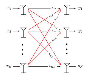
Fig. 2. The K-user GIC. User i for  $i \in \{1, 2, ..., K\}$  wishes to communicate with its corresponding receiver while receiving interference from other users.
