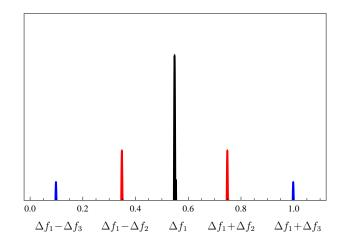
Figure 5: Expected structure for a "true" signal (arbitrary units). The black peak at the frequency  $\Delta f_1$  is the signal. Our leakage monitoring leads to sidebands at frequencies  $\Delta f_1 \pm \Delta f_2$  (red) and  $\Delta f_1 \pm \Delta f_3$  (blue) which are hopefully much smaller.
