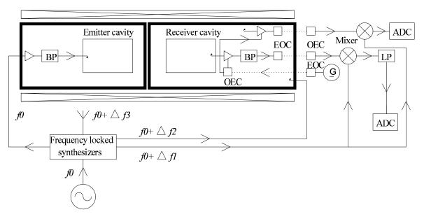
Figure 6: Setup for an experiment suitable for axion like particle detection. A solenoid provides for the required strong magnetic field.
