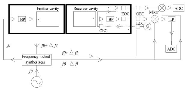
Figure 4: Setup of the experiment with "test signals" at slightly different frequencies for leakage monitoring. For details see main text.
