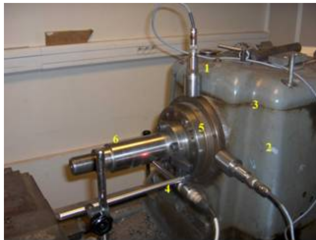
Figure 4 Position of transducers in acquisition schema to acquire vibrations of the spindle ERNAULT. 1- Accelerometer AS020 -vertical plan (V); 2- Accelerometer AS020 -horizontal plan (H), 3- Gearbox of Ernault HN400 lathe; 4- Tachometer; 5- Spindle bearing front side; 6- Work piece.
