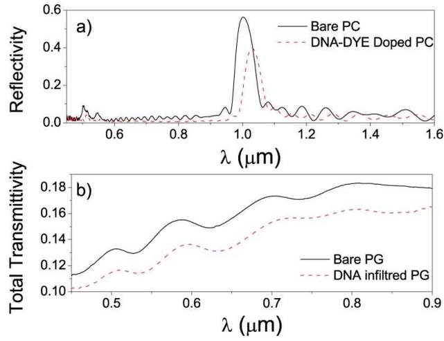
Fig. 3. (Color online). a) Reflectivity as function of wavelength measured for infiltrated (dashed line) and bare (continuous line) photonic crystal. The Bragg peak is evident around  $1 \mu\text{m}$  ; b) Total transmissivity as a function of wavelength in bare (continuous line) and DNA-filled (dashed line), photonic glass.
