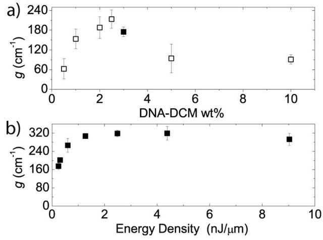
Fig. 2. Optical gain coefficient  $g$  plotted as function of DNA-DCM weight percentage (a) and of pump pulse energy density (b) for a DNA to DCM ratio of 3 wt% (black dot in fig 2a).
