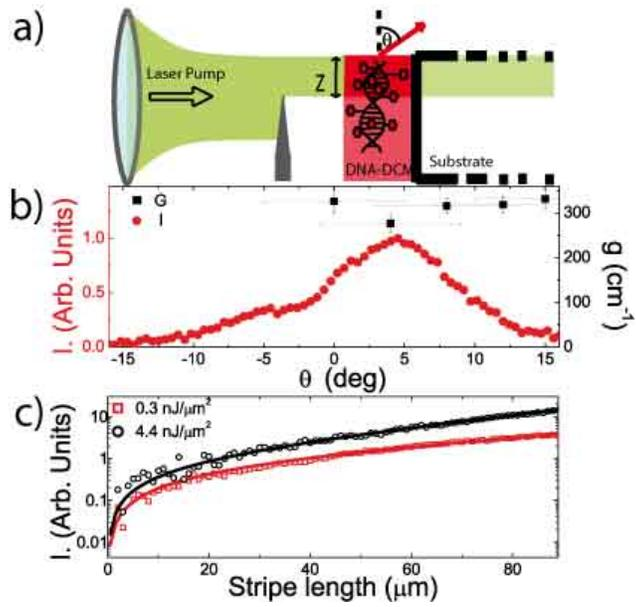
Fig. 1. (Color online). a) VSL setup; b) Intensity from the illuminated stripe (solid circles) and optical gain coefficient  $g$  (solid squares) as function of the detection angle  $\theta$ ; c) VSL measurement at two different pump energies. The continuous lines are fit from the model (see text).
