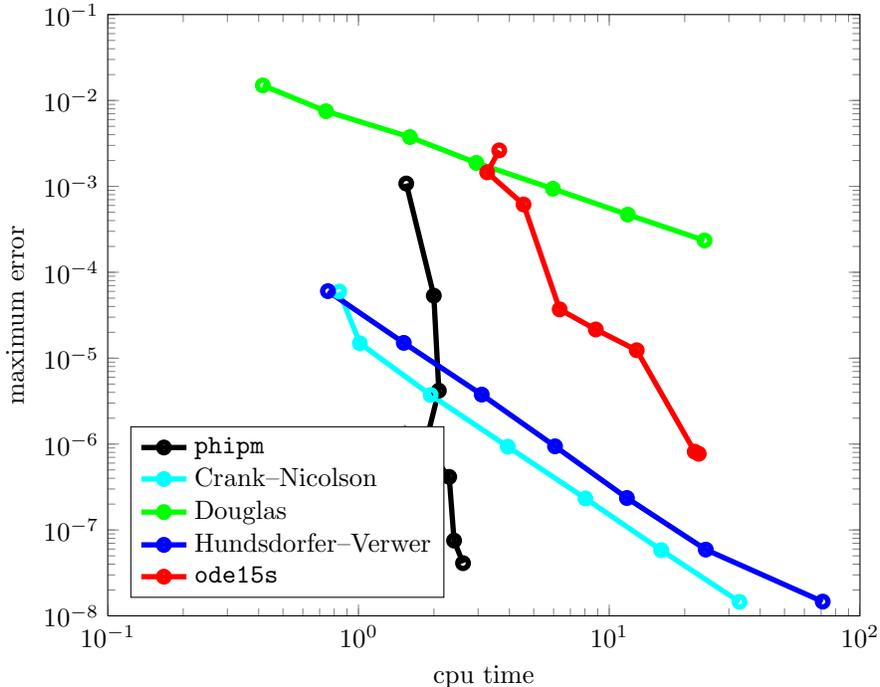
FIGURE 1. Plots of maximum error (on the domain  $[0, 2K] \times [0, 1]$ ) against CPU time for the system of ODEs from the discretized Heston PDE. The two ADI schemes are the represented by the: green line (Douglas); blue line (Hundsdorfer and Verwer), the cyan line is Crank-Nicolson, the red line is `ode15s` and the black line is `phipm`.
