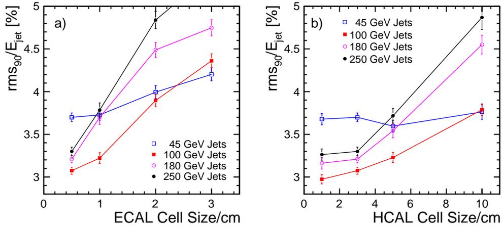
Figure 13: **a)** the dependence of the jet energy resolution ( $rms_{90}$ ) on the ECAL transverse segmentation (Silicon pixel size) in the LDCPrime model. **b)** the dependence of the jet energy resolution ( $rms_{90}$ ) on the HCAL transverse segmentation (scintillator tile size) in the LDCPrime model. The resolutions are obtained from  $Z \rightarrow u\bar{u}, d\bar{d}, s\bar{s}$  decays at rest. The errors shown are statistical only.
