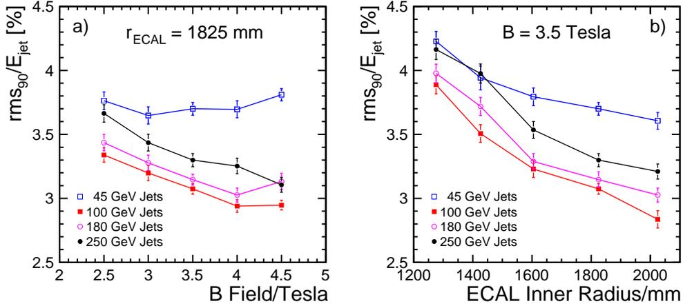
Figure 12: **a)** the dependence of the jet energy resolution ( $rms_{90}$ ) on the magnetic field for a fixed ECAL inner radius. **b)** the dependence of the jet energy resolution ( $rms_{90}$ ) on the ECAL inner radius a fixed value of the magnetic field. The resolutions are obtained from  $Z \rightarrow u\bar{u}, d\bar{d}, s\bar{s}$  decays at rest. The errors shown are statistical only.
