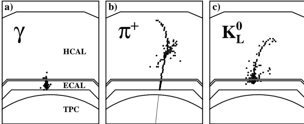
Figure 2: Example simulated single particle interactions in the ILD detector concept: a) a 10 GeV photon; b) a 10 GeV  $\pi^+$  and c) a 10 GeV  $K_L^0$ . Hits in the TPC, ECAL and HCAL are shown. For the ECAL (HCAL) all hits with energy depositions  $> 0.5$  ( $0.3$ ) minimum ionising particle equivalent are displayed. Simulated TPC hits are digitised assuming 227 radial rows of readout pads.
