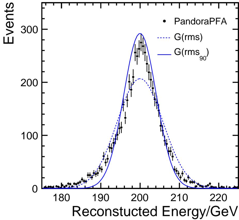
Figure 7: The total reconstructed energy from reconstructed PFOs in 200 GeV  $Z \rightarrow uds$  events for initial quark directions within the polar angle acceptance  $|\cos \theta_{q\bar{q}}| < 0.7$ . The dotted line shows the best fit Gaussian distribution with an rms of 5.8 GeV. The solid line shows a Gaussian distribution, normalised to the same number of events, with standard deviation equal to  $\text{rms}_{90}$  (*i.e.*  $\sigma = 4.1$  GeV).
