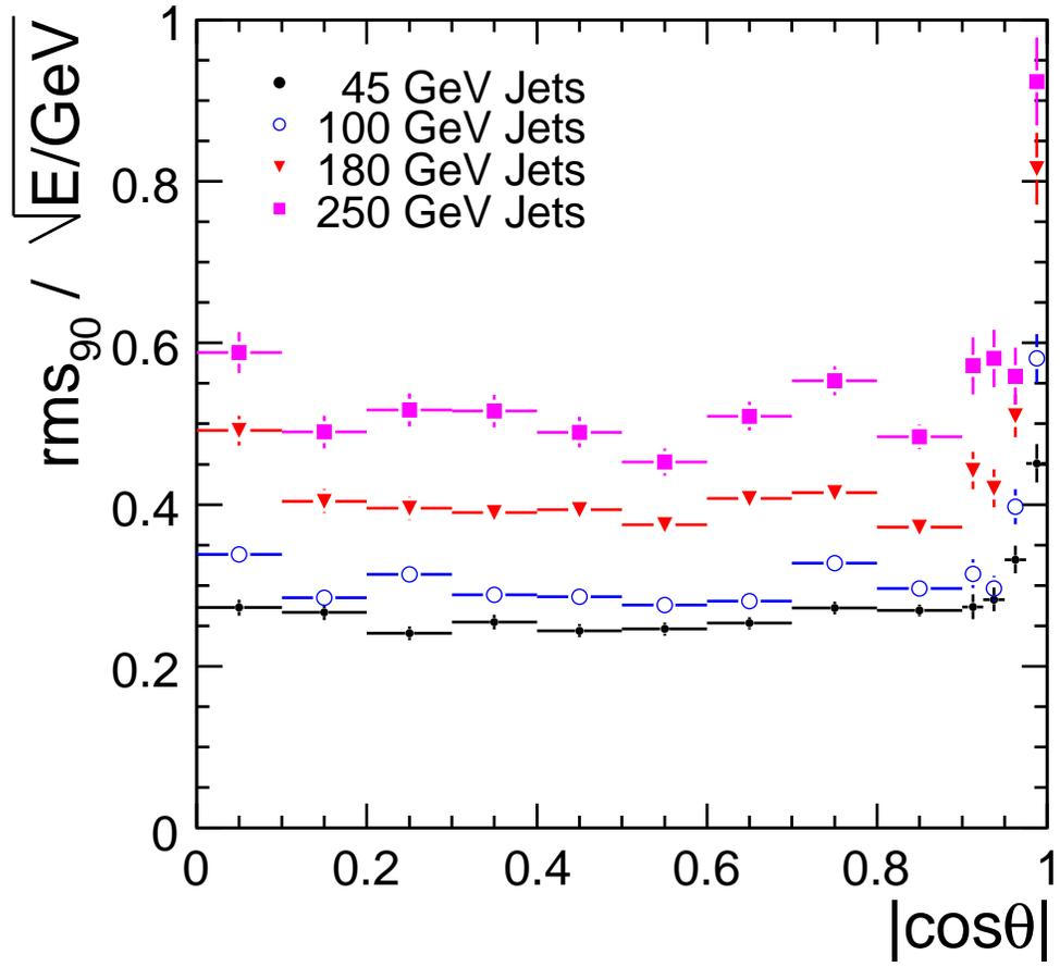
Figure 8: The jet energy resolution, defined as the  $\alpha$  in  $\sigma_E/E = \alpha/\sqrt{E(\text{GeV})}$ , plotted versus  $\cos\theta_{q\bar{q}}$  for four different values of  $\sqrt{s}$ . The plot shows the resolution obtained from  $(Z/\gamma)^* \rightarrow q\bar{q}$  events ( $q=u,d,s$ ) generated at rest.
