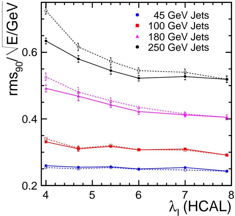
Figure 11: Jet energy resolutions ( $\text{rms}_{90}$ ) for the LDCPrime as a function of the thickness (normal incidence) of the HCAL. In addition, the ECAL contributes  $0.8\lambda_I$ . Results are shown with (solid markers) and without (open markers) taking into account energy depositions in the muon chambers. All results are based on  $Z \rightarrow u\bar{u}, d\bar{d}, s\bar{s}$  with generated polar angle in the barrel region of the detector,  $|\cos\theta_{q\bar{q}}| < 0.7$ .
