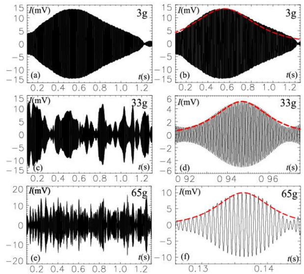
FIG. 2: Waveforms of the bandpass-filtered signals ( $f = 1.6 \pm 0.2$  kHz) of the first (sub)harmonic measured at different acceleration levels: (a,b)  $\Delta A = 3g$ ; (c,d)  $\Delta A = 33g$ ; (e,f)  $\Delta A = 65g$ . Dashed lines in (b,d,f) correspond to the  $\text{sech}(t)$  fit of the wavelet envelopes.
