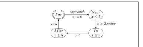
Fig. 2. A timed automaton modelling the position of a train with respect to a gate. The train alterns between locations Far, Near, In, After. When transition labelled by *approach* is taken, clock x is reset to 0. When clock x becomes greater than 2, transition labelled by *enter* can be taken. The train must leave locations Near, In, After before clock x becomes greater than 5.
