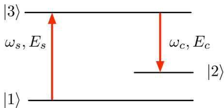
FIG. 1:  $\Lambda$ -three level system with two ground states and one excited state. A transition from state  $|1\rangle$  to  $|3\rangle$  can be performed with a SIT soliton. The transition from  $|2\rangle$  to  $|3\rangle$  can be performed with control light field. A radiative transition between  $|1\rangle$  and  $|2\rangle$  is dipole forbidden.
