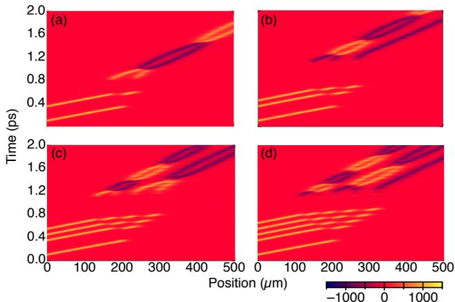
FIG. 7: The electric field  $E_S$  ( $\text{Vm}^{-1}$ ) throughout the medium in a set of calculations where two (a), three (b), four (c), and five (d) SIT solitons are trapped in the medium. Subsequently, from  $t=0.8$  ns, a continuous wave control field is launched into the medium that interacts with the ground state coherence structure to form sets of bi-solitons and single solitons which propagate in the  $+z$ -direction.
