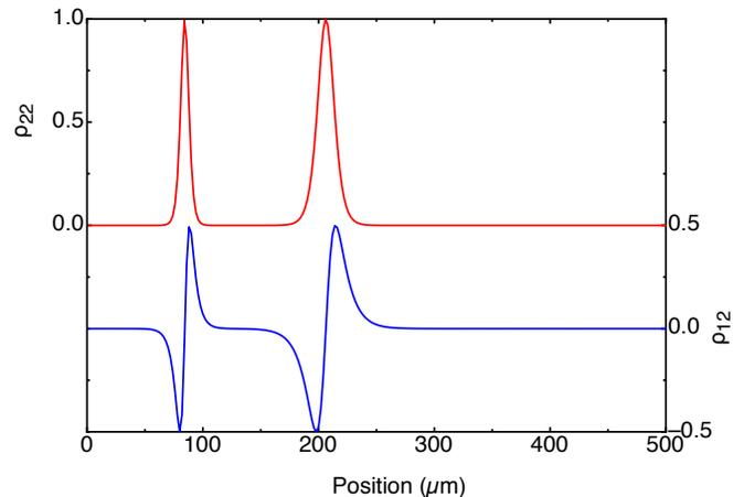
FIG. 6:  $\rho_{22}$  (red trace) and ground state coherence (blue trace) through out the medium after two SIT solitons are captured. In this case, the peak intensity of the first SIT soliton is less than that of the second.
