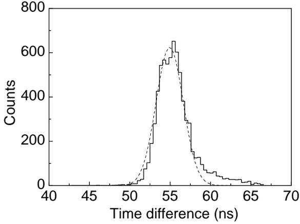
Fig. 2. The distribution of the time difference between the RPC and the master trigger.
