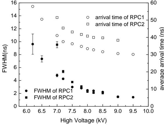
Fig. 3. The time resolution (FWHM) and the average signal arrival time with respect to the master trigger as a function of HV for two silicon coated RPC.
