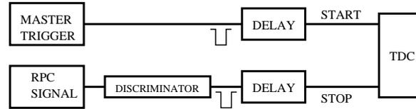
Fig. 1. Schematic representation of the time resolution measurement setup. A common start Phillips Scientific 7186 Time to Digital Converter (TDC) was used.
