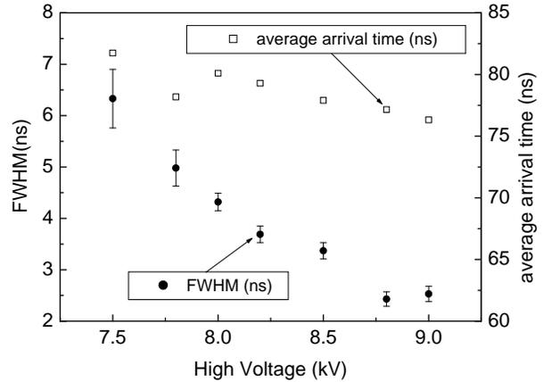
Fig. 5. The time resolution (FWHM) and the average signal arrival time of one RPC with respect to another RPC as a function of HV.
