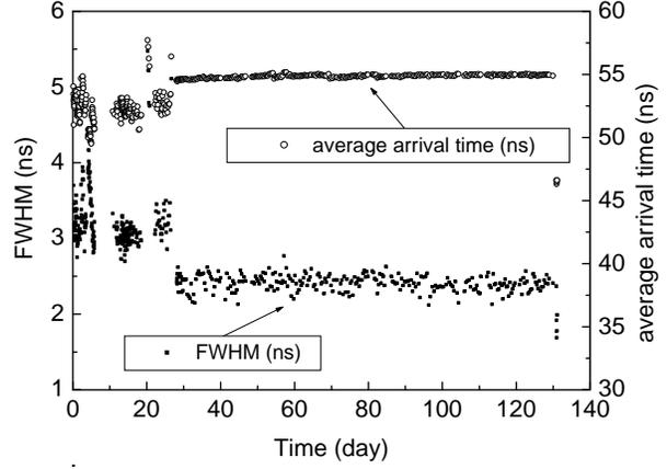
Fig. 4. The time resolution (FWHM) and the average signal arrival time as a function of period of operation.
