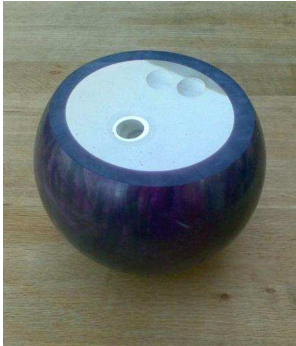
Figure 1. The physical rock'n'roller, constructed by slicing off a polar cap from a standard bowling ball. The polar angle is \Theta \approx 53^\circ .
