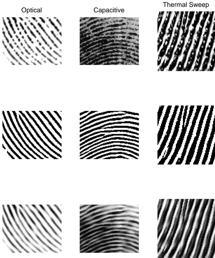
Figure 4: In the left column, we show results on an image captured by an optical sensor, and in the middle column, by a capacitive sensor, and in the right column, by a thermal sweep sensor. We show results in the selected subregions of the images. The top row shows the original images, the middle row shows the binarized images and the bottom row shows the enhanced images.
