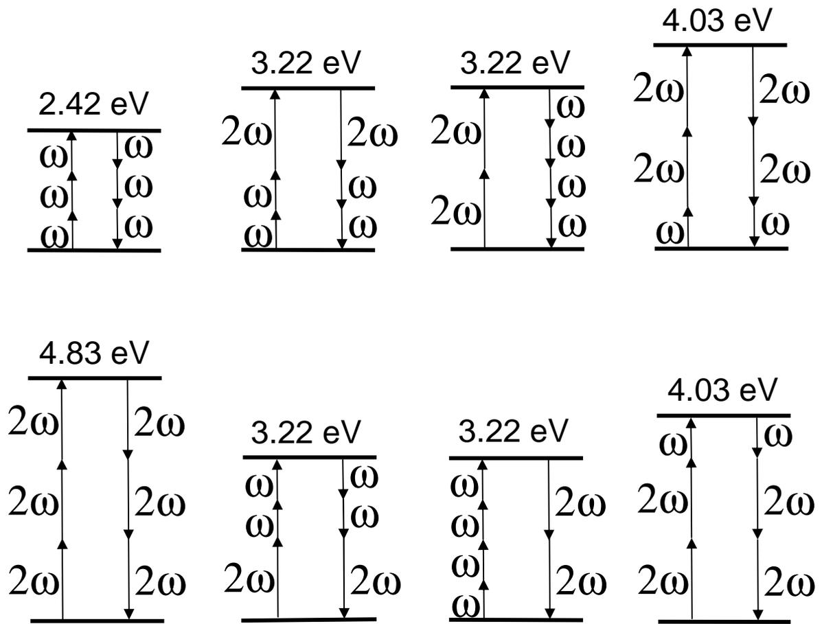
Fig. 4 Diagrams of quintic self- and cross-phase and frequency mixing transitions.
