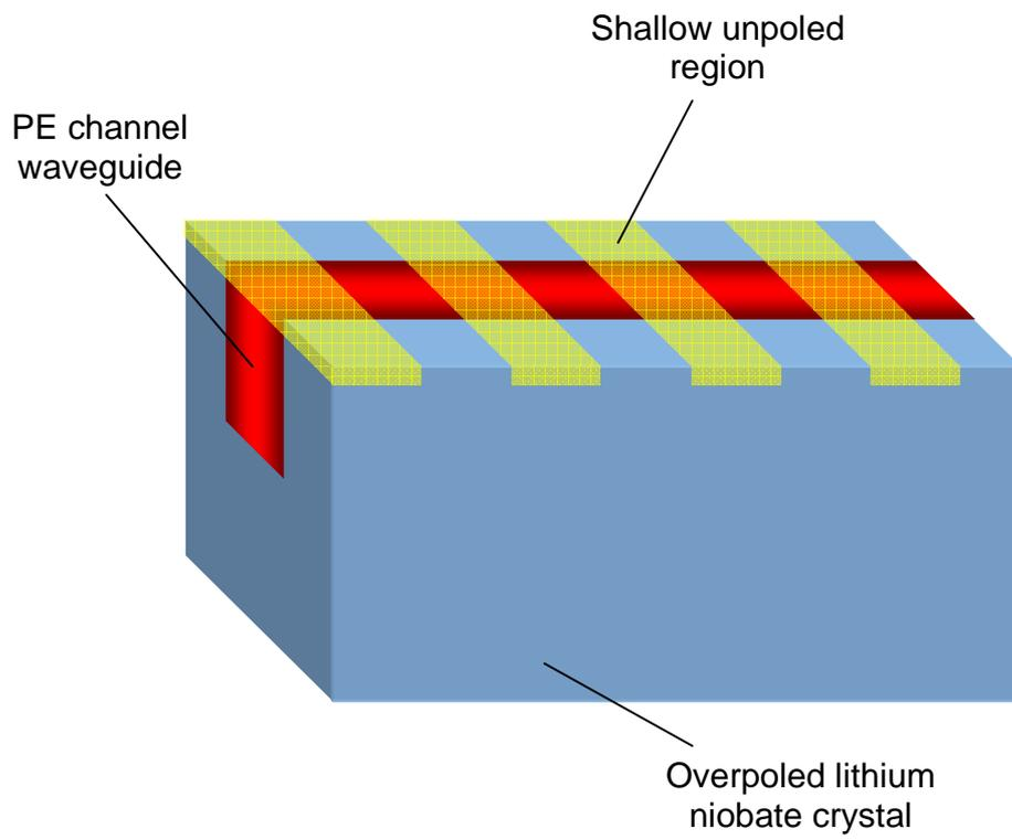
Fig. 1 Sketch of the nonlinear waveguide. The LN crystal is poled everywhere but retains a shallow periodic pattern that doesn't reach the whole PE channel depth.
