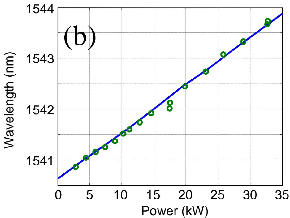
Fig. 2 (a) Measured (open circles) and predicted (solid line) maximum SHG efficiency versus launched FF peak power. (b) Measured (open circles) and predicted (solid line) wavelength shift. Nonlinear absorption is not included in the model.
