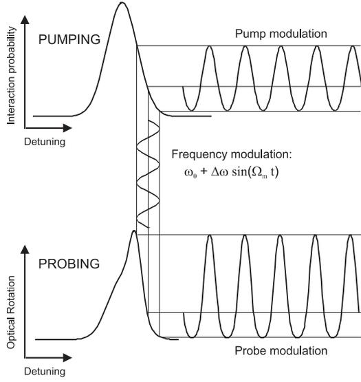
FIG. 8: Illustration of the time-dependent optical pumping and optical rotation generated via frequency modulation for high light power (where alignment-to-orientation is the dominant cause of optical rotation, causing enhanced rotation for  $F \rightarrow F + 1$  transitions with the same sign as compared to  $F \rightarrow F - 1, F$  transitions, see text).
