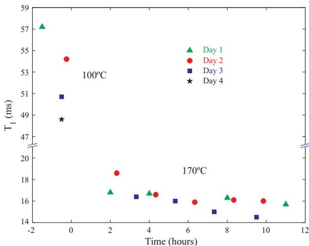
FIG. 2: (Color online) Measurements of the polarization lifetime  $T_1$  taken in an OTS-coated rubidium cell (#13) with 10 Torr of nitrogen quenching gas, showing degradation of the coating after extended operation at 170°C. Note that at 170°C the relaxation time is dominated by collisions between rubidium atoms, indicating that the surface coating is sufficiently effective.
