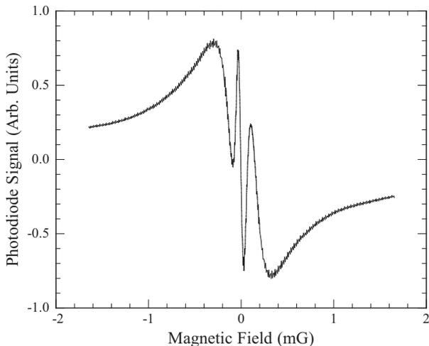
FIG. 4: A dispersion curve with amplitude of 1.6 radians measured in a coated cell (#11); rotations larger than  $\pi/4$  radians cause the polarimeter signal to turn over.
