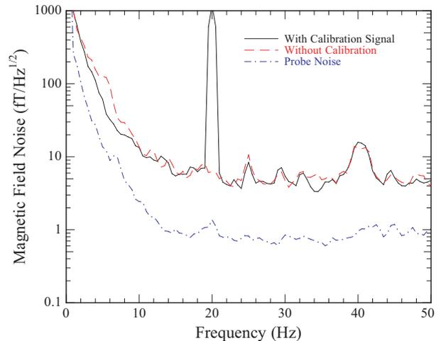
FIG. 5: (Color online) Single-channel noise spectrum taken at 150°C in a coated potassium cell without quenching gas, showing sensitivity of  $6 \text{ fT}/\sqrt{\text{Hz}}$ , possibly limited by the noise of the magnetic shielding. The optical noise of the probe beam was measured in the absence of pumping light, so that the vapor was unresponsive to ambient field noise.
