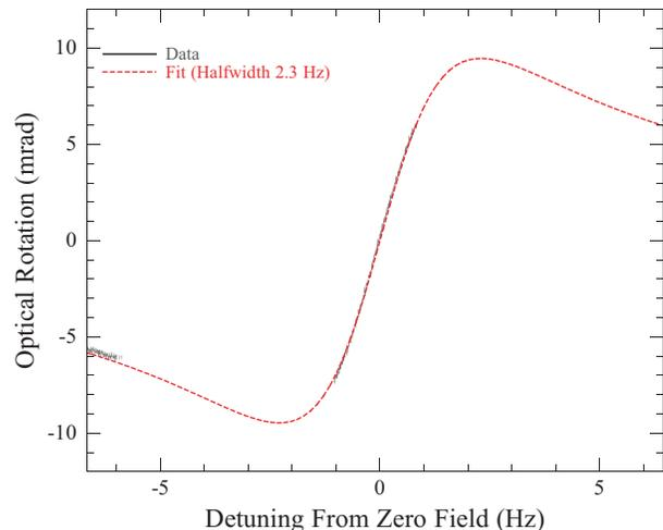
FIG. 3: (Color online) A narrow magnetometer resonance signal obtained in the SERF regime with an OTS-coated cell (#7) and very low optical pumping rate, fitted to a Lorentzian with HWHM of 2.3 Hz.
