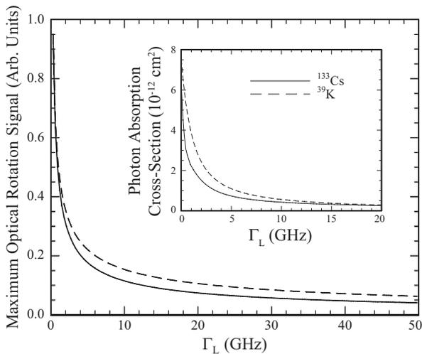
FIG. 1: Scaling of the maximum optical rotation signal  $\theta(\nu)e^{-n\sigma(\nu)l}$  of the probe beam, taken at optimal detuning from resonance, as a function of buffer gas pressure broadening (FWHM)  $\Gamma_L$ . The potassium and cesium curves are normalized separately, and  $\Gamma_G$  is set to its value at 160°C. The inset shows the maximum photon absorption cross-section as a function of  $\Gamma_L$ .
