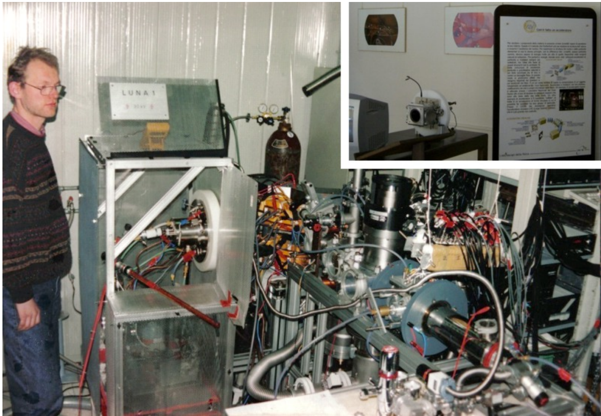
Figure 5: Photo of the LUNA I accelerator. On the left side one sees the ion source with the acceleration drift and on the right side the gas target with a beam calorimeter at the end. The inset (upper right corner) shows the accelerator part now displayed in a museum at Teramo, Italy.
