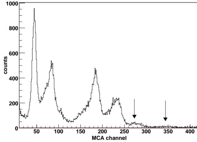
Figure 9: Spectrum of low the  $^{241}\text{Am}$  low energy gamma lines, obtained with the alphas blocked: 3.0 keV and 6.1 keV fluorescences; 13.9 keV, 17.7 keV and 21.0 keV X-rays; 26.4 keV gamma lines from  $^{241}\text{Am}$
