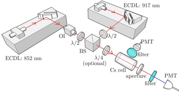
Fig. 2. Schematic of experimental arrangement. Two lasers (852 nm, 917 nm) excite  $^{133}\text{Cs}$  on the 6S-6P-6D transitions, and coherent 455 nm radiation is emitted. The blue beam is sent through an aperture and a band-pass filter and is detected with a photomultiplier tube (PMT). A PMT is also used to measure the blue fluorescence in the cell. OI is an optical isolator, and BS is a non-polarizing beam splitter.
