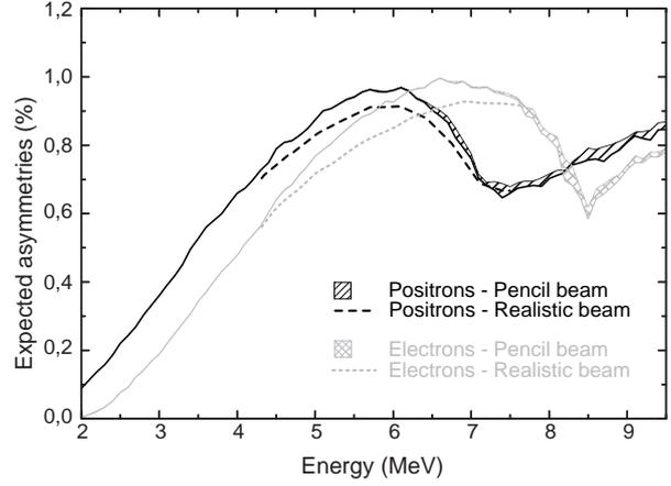
Figure 42: Simulations of the asymmetries  $\delta$ , Eq. (8), of the energies observed in the central CsI crystal on reversal of the polarity of magnet TP1 as a function of positron/electron energy for the experimental beam and for a pencil beam.
