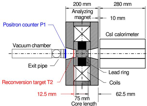
Figure 23: Sketch of the positron polarimeter. Positrons entered from the left, passing in succession through the exit window of the spectrometer, the Si-W counter P1, the reversion target T2, after which the reconverted photons passed through the iron-core magnet TP1 and were absorbed in the CsI calorimeter on the right.
