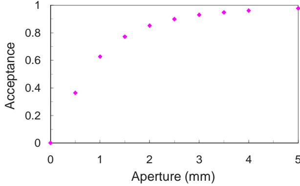
Figure 45: Simulated acceptance of the collimator C2 as a function of the collimator aperture, assuming that the photon beam axis and the collimator axis coincided.
