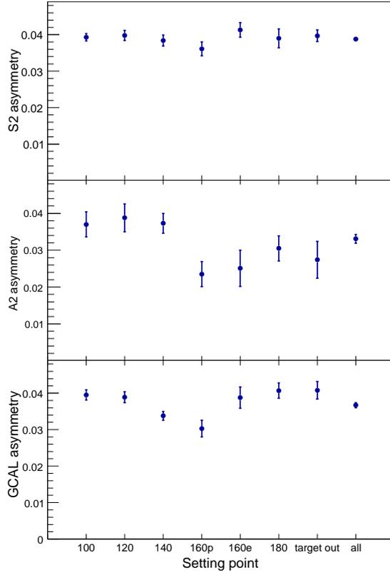
Figure 57: The average asymmetry  $\delta$  observed in the photon detectors S1, A1, and GCAL in the seven data segments (Table 4) of the experiment, as well as the asymmetries averaged over the entire experiment.
