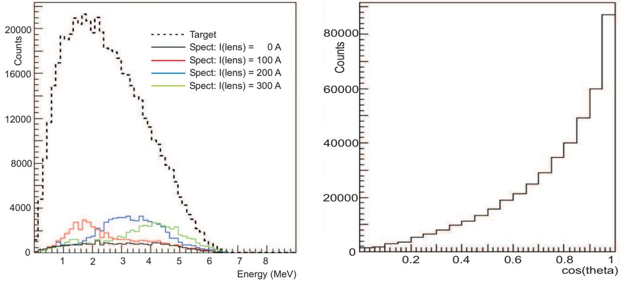
Figure 37: Simulations of focusing of positrons by the solenoid lens SL. *Left:* The energy spectra of positrons emerging from the production target T1 and of positrons entering the spectrometer D2 for different solenoid currents. *Right:* The polar angle distribution,  $\cos \theta$ , of positrons at the target exit surface.
