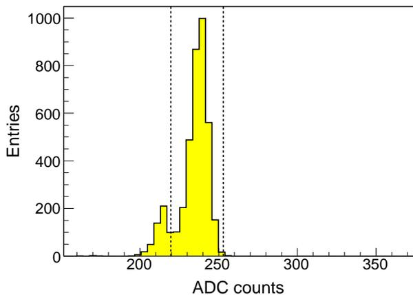
Figure 58: Example of a distribution of the beam current in toroid BT (see Fig. 2) that shows a fluctuation to low current. Only events with current within the  $\pm 3\sigma$  cuts about the mean were used in the subsequent analysis.
