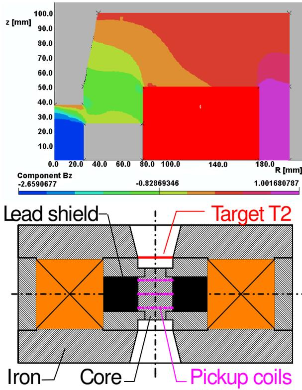
Figure 24: Top: 2d-field model in the  $r$ - $z$  plane of magnet TP1. Bottom: Horizontal section of magnet TP1 showing the location of the pickup coils. The top figure corresponds to the first quadrant of the bottom figure.
