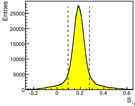
Figure 60: The distribution of renormalized, background-subtracted energies  $S_{ij}$ , defined in Eq. (24), in the central CsI crystal for a typical data cycle. The dotted lines indicate the  $\pm 2\sigma$  fit range described in the text.
