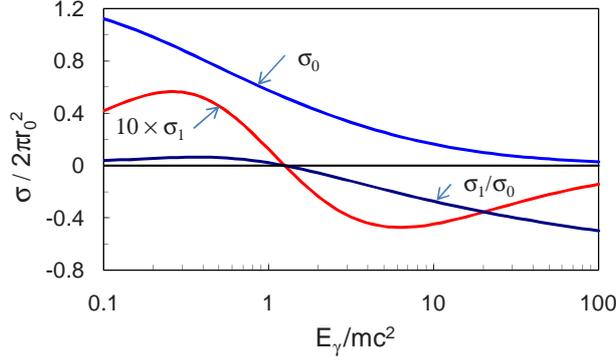
Figure 8: The total cross sections  $\sigma_0$  and  $\sigma_1$  of Eq. (5) for Compton scattering of longitudinally polarized photons of energy  $E_\gamma$  off unpolarized and longitudinally polarized electrons, respectively;  $r_0$  is the classical electron radius.
