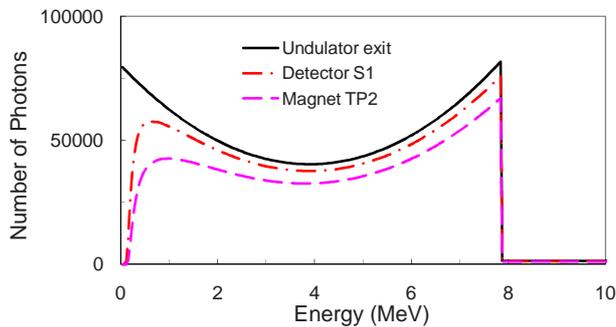
Figure 43: Simulated photon spectra  $N_\gamma(E)$  at the exit of the undulator, at detector S1, and incident on polarimeter magnet TP2.
