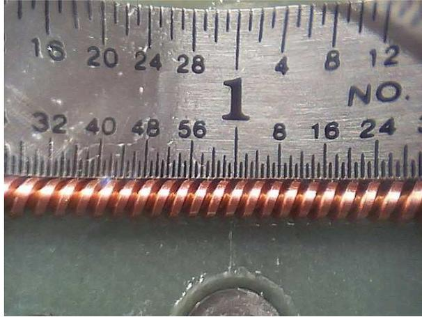
Figure 13: Photograph of the windings of undulator U1. The rectangular cross-section wire has dimensions of  $0.6 \times 0.6 \text{ mm}^2$ , and a period of 2.54 mm. The smallest scale division is  $1/64$  of an inch (0.397 mm).
