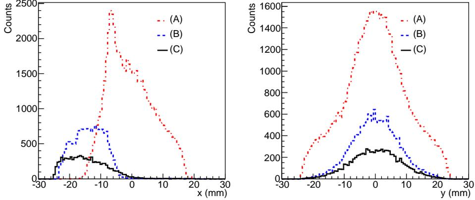
Figure 39: Simulated distributions of positrons along the  $x$ - and  $y$ -axis at the exit of the spectrometer D2 (A), at the detector P1 (B) and at the reconversion target T2 (C) for spectrometer current 140 A.
