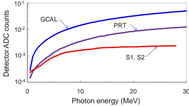
Figure 46: GEANT3 simulation of the single-photon response  $R(E)$  of the  $\gamma$ -detectors S1/S2, GCAL, and PRT.
