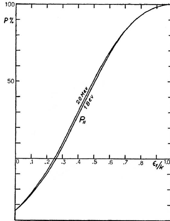
Figure 5: Longitudinal polarization of positrons (or electrons) produced by conversion of monochromatic circularly polarized photons in an infinitely thin target, as a function of the ratio  $E_{e^+}/E_{\gamma}$  of positron to photon energies; from [4].
