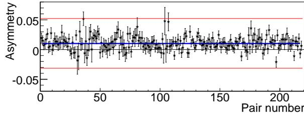
Figure 61: The asymmetries  $\delta_k$  observed for the 218 cycles pairs in the positron polarimeter for  $I_S = 140$  A during the second running period. Also shown is the best-fit  $\delta = \langle \delta_k \rangle$  (horizontal blue line) and the  $\pm 3\sigma$  band used for the cut on outliers.
