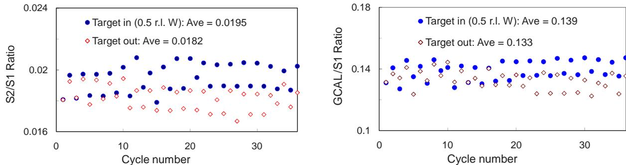
Figure 54: Transmission of undulator photons through magnet TP2 as measured with detectors S2 (left) and GCAL (right), both normalized to detector S1.
