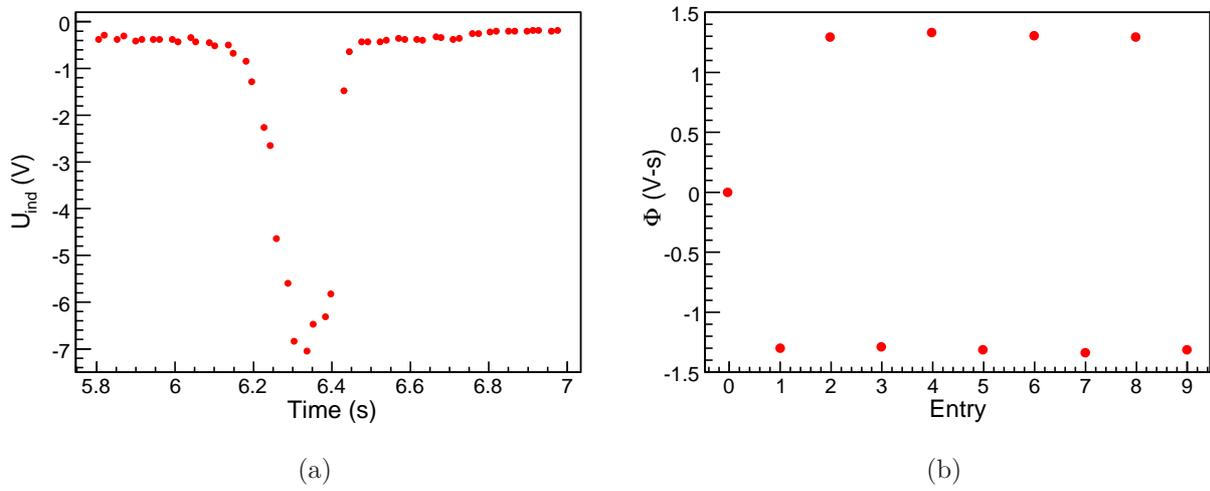
Figure 26: Induced-voltage signal upon field reversal in one of several pickup coils surrounding the iron core of magnet TP1: (a) voltage vs. time (left); (b) Magnetic flux  $\Phi = \int V dt = BA$  for several polarity flips (right).
