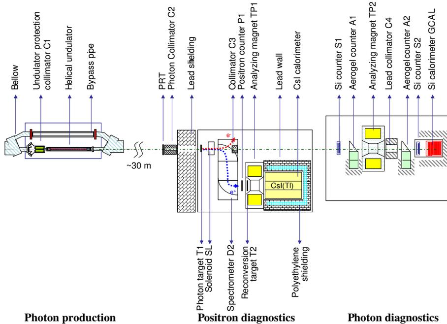
Figure 11: Schematic of the experimental apparatus along the  $\gamma$ -line, including photon production in the undulator, conversion to  $e^\pm$  in target T1, and subsequent diagnostics of photons and positrons. During the initial setup of the electron beam the bypass pipe was placed in the beamline rather than the undulator.
