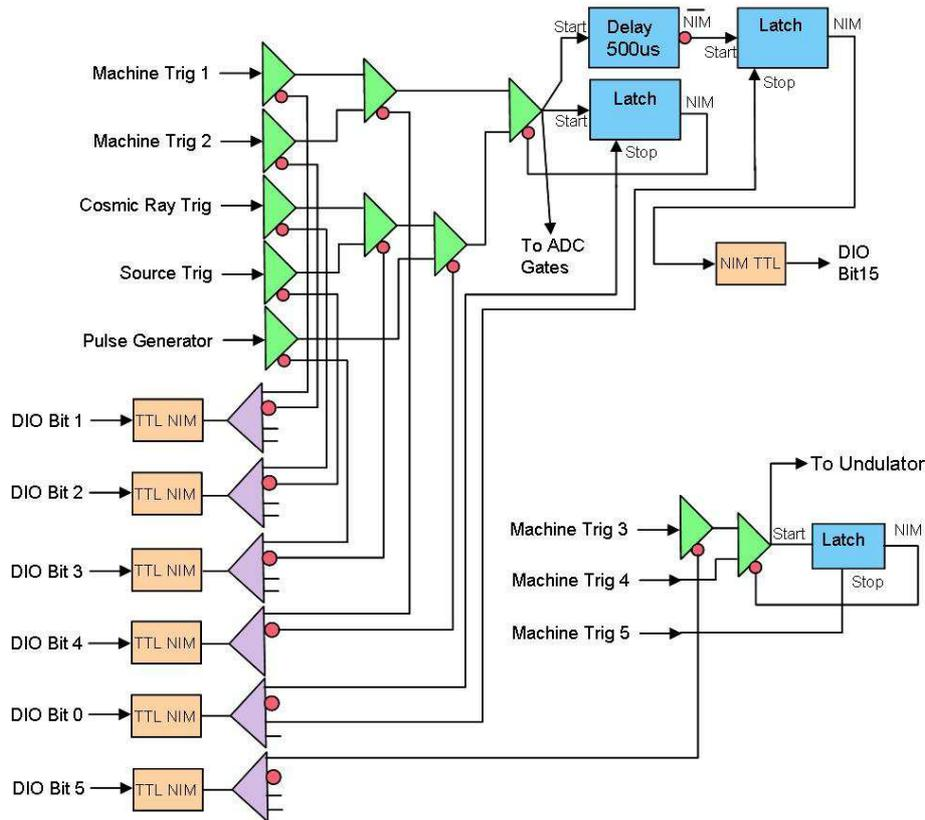
Figure 34: Trigger logic
