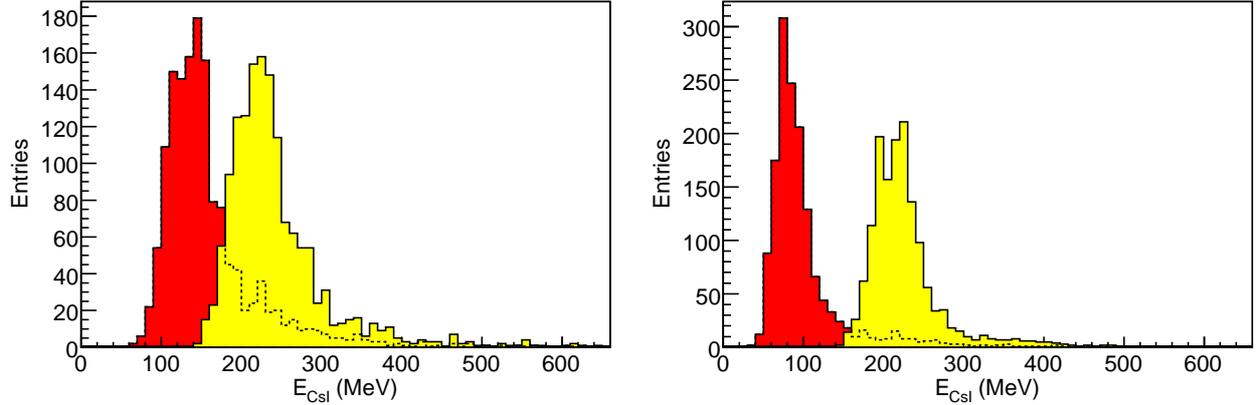
Figure 59: Two examples of energy distributions for events in the central CsI crystal, taken with spectrometer current  $I_S = 160$  A; (left) positrons, (right) electrons. Within each plot the left histogram is for undulator off (out of time) and the right histogram is for undulator on.
