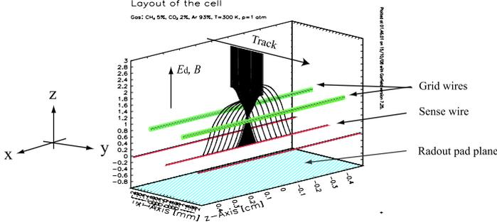
Figure 3: Simulated drift electron paths without diffusion in TDR gas for a track perpendicular to the wires ( $B = 4$  T).
