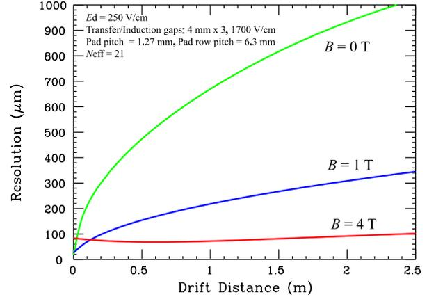
Figure 8: Expected resolution of a GEM-based TPC operated in T2K gas for tracks perpendicular to the pad rows.
