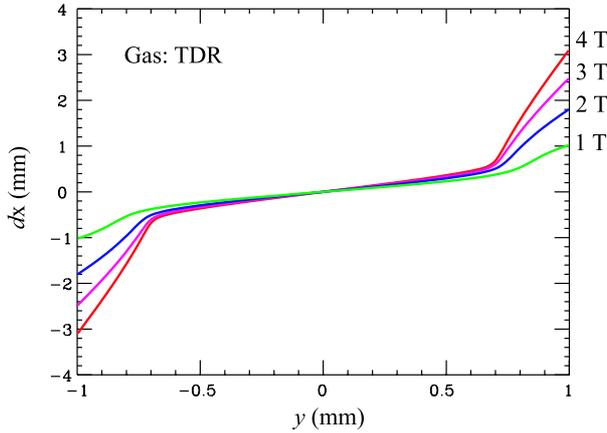
Figure 4: Displacement of the arrival position of drift electrons on the sense wire as a function of the initial position along the track for  $B = 1, 2, 3$  and  $4$  T. The coordinate  $y$  is measured from the point on the track right above the sense wire. The increase of displacement ( $dx$ ), especially for large  $y$ , degrades the spatial resolution significantly.
