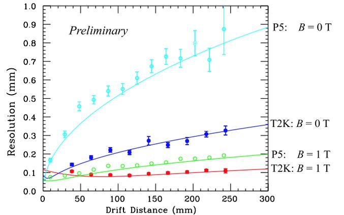
Figure 6: Spatial resolution as a function of the drift distance obtained with a T2K gas ( $E_d = 250$  V/cm) for  $B = 0$  and  $1$  T. The resolutions obtained in the beam test with a P5 gas ( $E_d = 100$  V/cm) are also shown for comparison.
