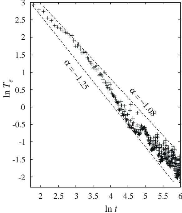
Fig. 1. Simulated electron temperature as function of time in the logarithmic scale. The inclined dashed lines show the power-like dependences  $T_e \propto t^\alpha$ ; the values of  $\alpha$  being presented near the respective lines.
