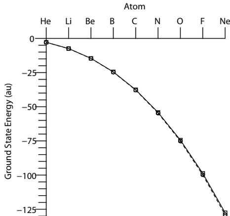
Figure 1: Experimental (dashed) and minimal asymptotics-based CI (solid) ground state energies of atoms.
