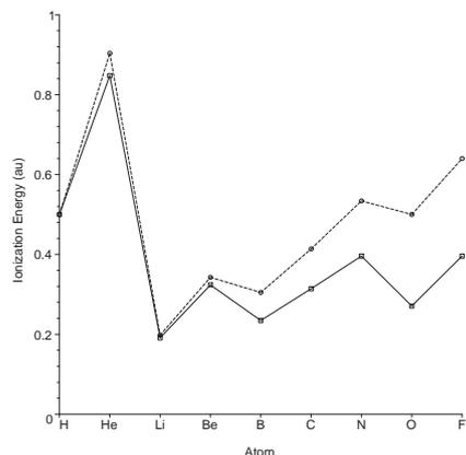
Figure 3: Experimental (dashed) and minimal CI (solid) ionization energies.
