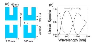
Fig. 1. (a) Schematic drawing of a square lattice of gold split-ring resonators. The thickness of the gold film is 25 nm. (b) Its linear spectra under a *x*-polarized normal incidence.
