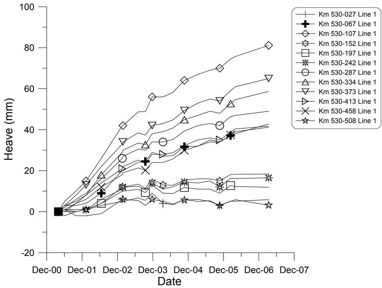
Figure 6. Heave observed on the leg of the catenary poles of the Line 1 from April 2001. (after SNCF, 2007).
