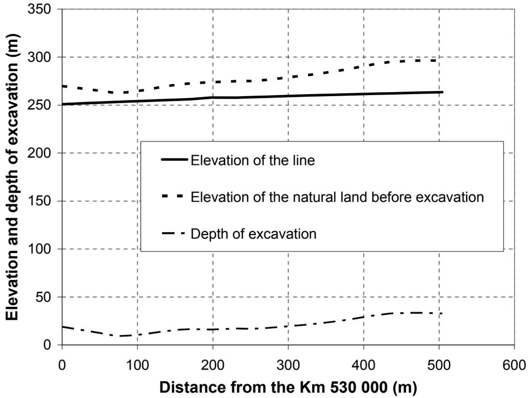
Figure 1. Elevations of the natural land (before excavation in 1998) and of the line (after excavation in 1998).
