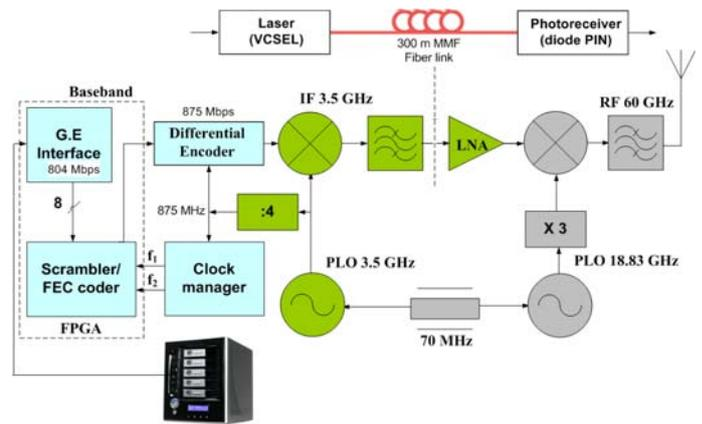
Figure 1. 60 GHz Wireless Gigabit Ethernet transmitter (Tx)
