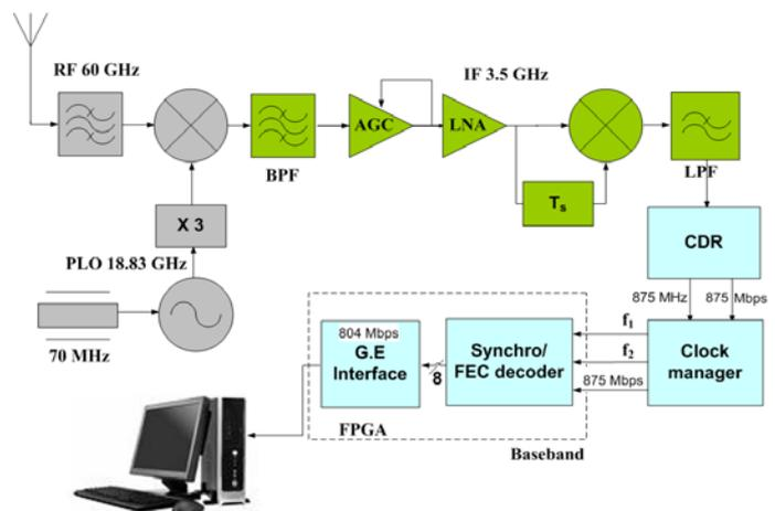
Figure 2. 60 GHz Wireless Gigabit Ethernet receiver (Rx)
