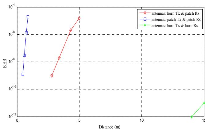
Figure 11. BER performance at 875 Mbps (without channel coding)
