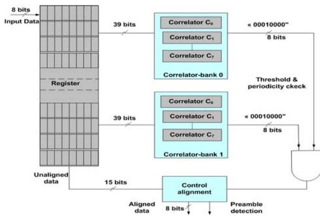
Figure 7. Preamble detection with periodicity and control alignment
