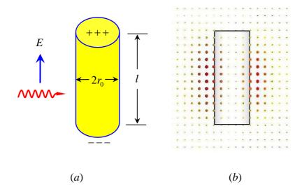
Figure 1: (a) Schematic view of the structure under study. The subwavelength gold nanorod is embedded in a dielectric, and the incident light is propagating with the electric field along the rod axis, thus exciting the longitudinal plasmon resonance. (b) The magnetic field distribution around the nanorod when a current flow in the rod is excited by the light electric field.
