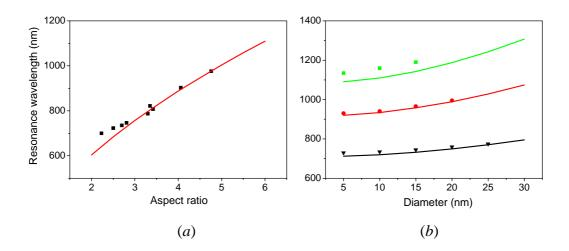
Figure 2: (a) Dependence of resonance wavelength on the aspect ratio. The squares represent the experimental data [10] and the line gives our calculated values (the rod diameter is fixed as 22nm). (b) Dependence of resonance wavelength on the rod radius. The symbols are obtained by numerical calculations [19] and the lines obtained by our calculation. Here the aspect ratio is set as 3, 5 and 7, respectively (from the bottom to the top).
