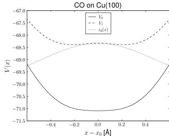
FIG. 5: Potential energy surfaces along the frustrated rotation mode of CO adsorbed on a Cu(100) surface. The coordinate  $x$  is a generalized coordinate representing the deviation from equilibrium.  $x = 0.4$  corresponds to a  $24^\circ$  angular deviation from the perpendicular position.
