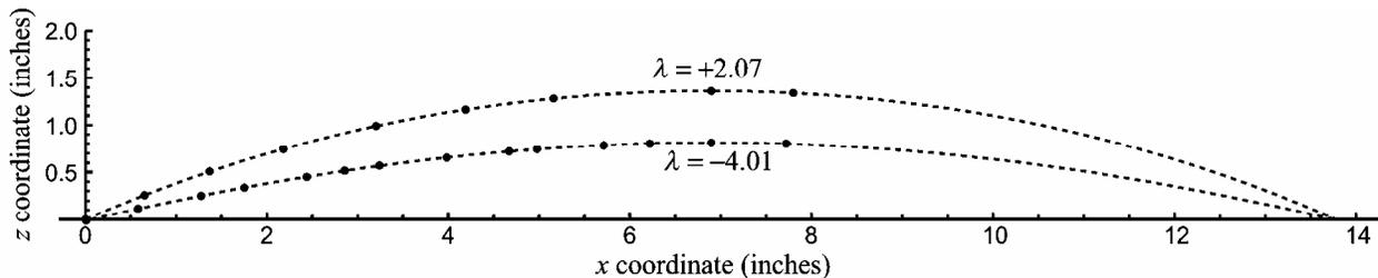
165 Figure 7, example inflation ( $\lambda = +2.07$ ) and deflation ( $\lambda = -4.01$ ) of a membrane showing
