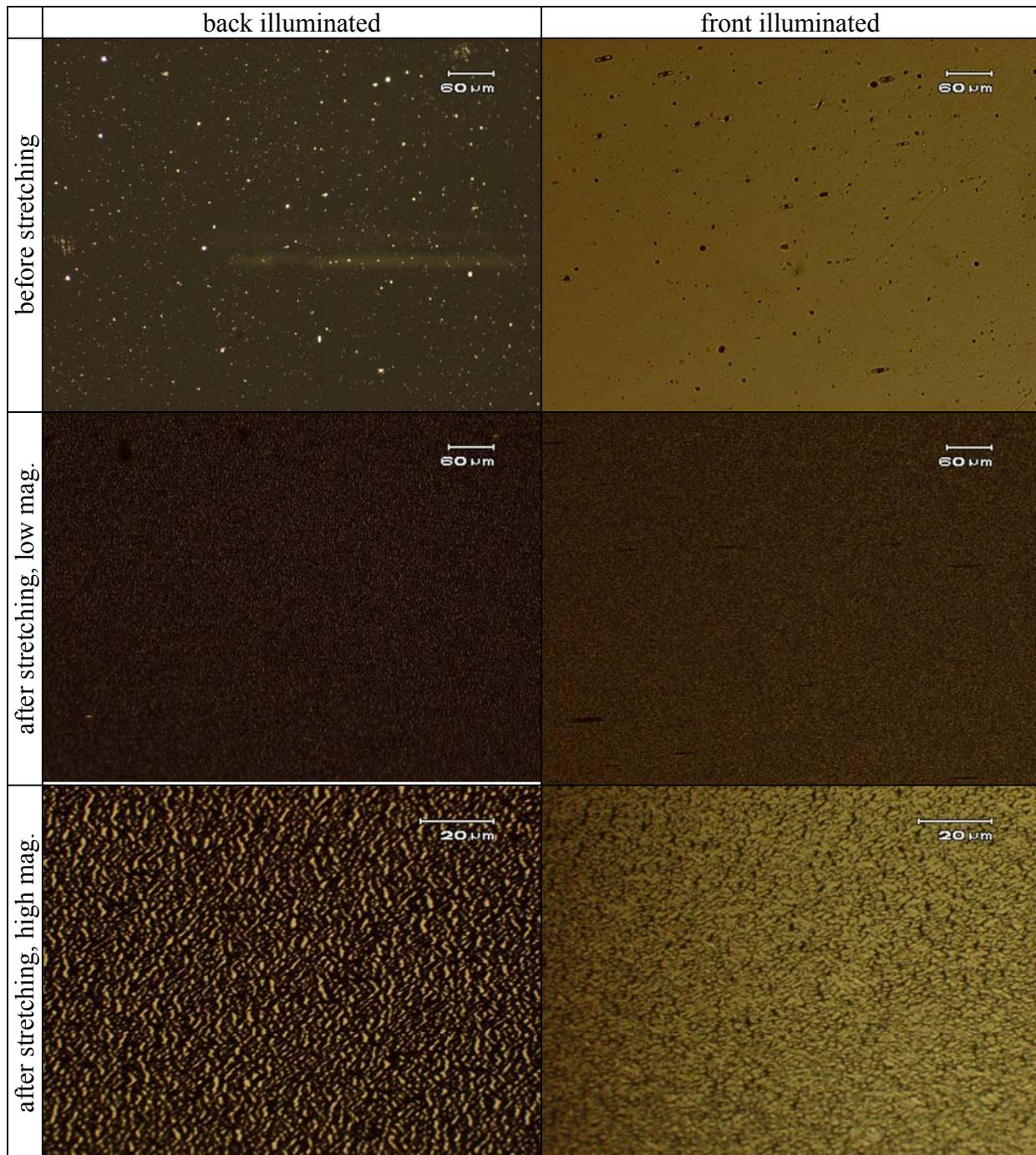
220 Figure 12, micrographs of aluminized Mylar before and after stretching about 200%: left column, back illuminated; right column, front illuminated; top row, before stretching; middle row, after stretching, low magnification; bottom row, after stretching, high magnification
