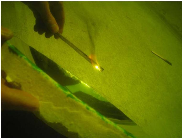
Figure 11, photograph of dish concentrating sunlight onto a wooden stick
