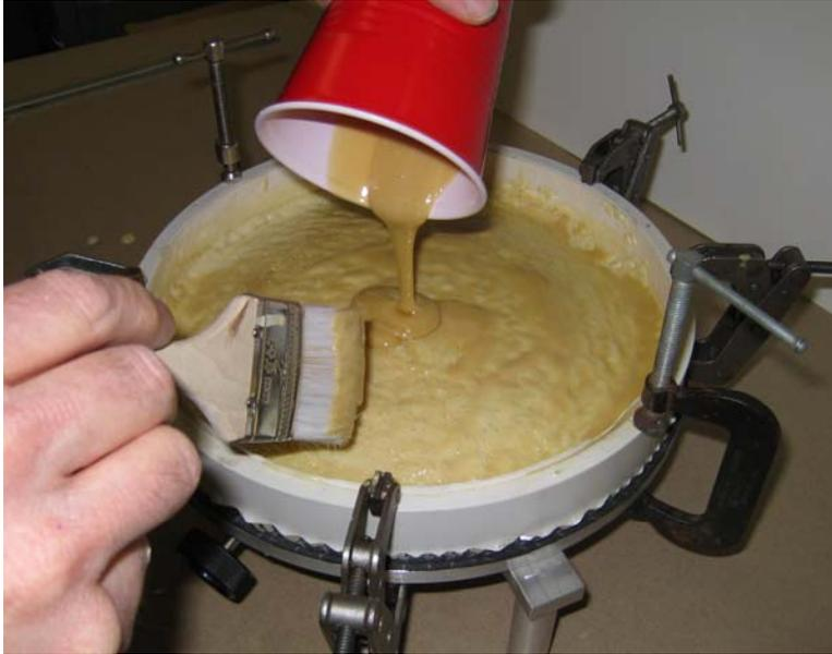
Figure 5, applying the fifth layer of foam
