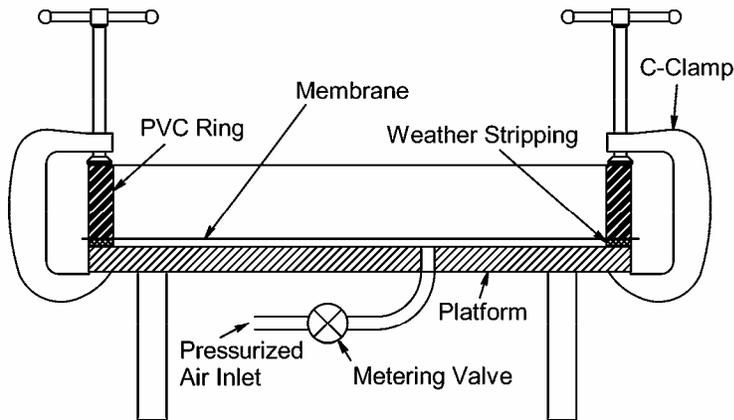
Figure 1, cross-section of the apparatus for making the dishes
