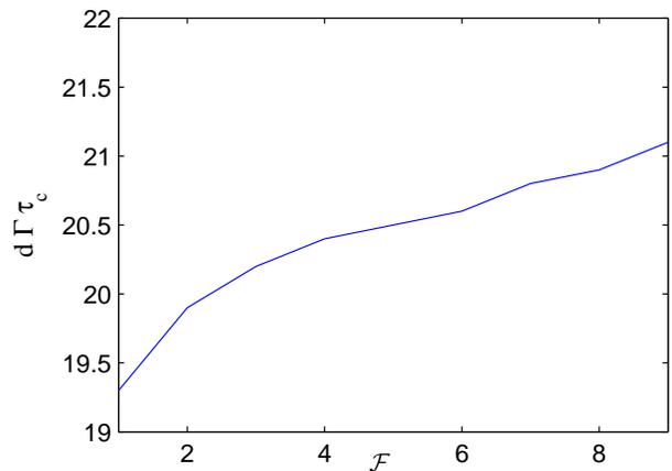
Figure 4: Plot of the time  $\tau_c$  measured in units of  $(d\Gamma)^{-1}$ , at which the intensity on the symmetry axis is dominated by SRS. The cross-over time is only weakly dependent on Fresnel number, and is given primarily by the optical depth.
