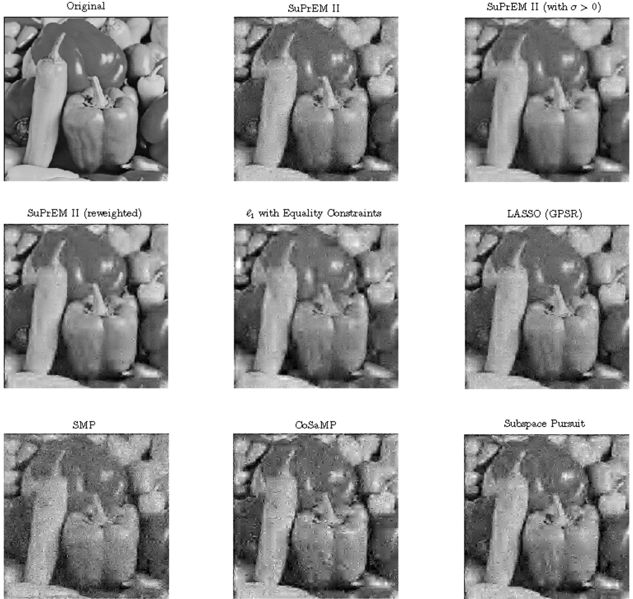
Fig. 6. Performance comparison of recovery algorithms with a 256 \times 256 natural image whose db2 wavelet coefficients are compressively sensed with N = 17000 measurements.
