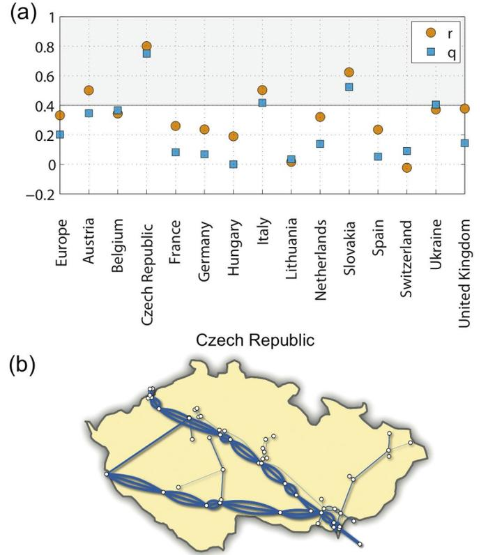
FIG. 5: (Colour online) (a) Pearson correlation coefficient,  $r$ , for the degrees of two linked nodes and the capacity of the linking pipeline; and percentage of capacity on parallel pipelines,  $q$ . We considered only countries with more than 50 pipelines. (b) Network layout for the Czech Republic. Link thickness is proportional to the pipeline capacity.
