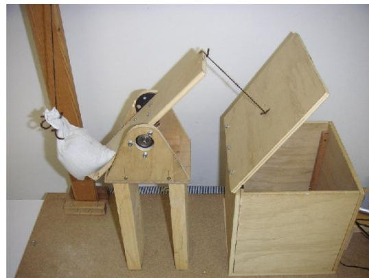
Fig.4 Here the sandbag has fallen, turned over the seesaw and opened the lid. In this photo taken during setup there is no balloon yet. The seesaw need not pull the lid up to the vertical. The balloon can be smaller than the box and come out sideways. Anyway, if the lid is pulled strongly enough at the beginning, it has enough momentum to move on up to vertical.
