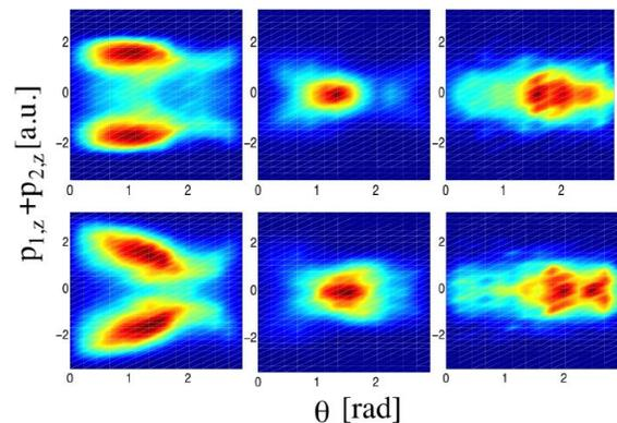
FIG. 4: Top panel corresponds to a laser pulse of  $10^{14}$  *Watts/cm*<sup>2</sup> and a 3-cycle duration; Bottom panel corresponds to a laser pulse of  $10^{14}$  *Watts/cm*<sup>2</sup> and a 3-cycle duration. From left to right we show the differential probability for the EI, RESI and DE mechanisms respectively.
