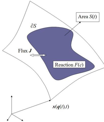
FIG. 1: A schematic diagram showing the flux of matter into, and out of a patch of area  $S$ . This flux comprises advective and diffusive parts, and is given by  $\mathbf{J} = \mathbf{U}c - \kappa \operatorname{grad}c$ , and  $d\ell$  is a line element on the curve formed by the boundary of the area  $S$ .
