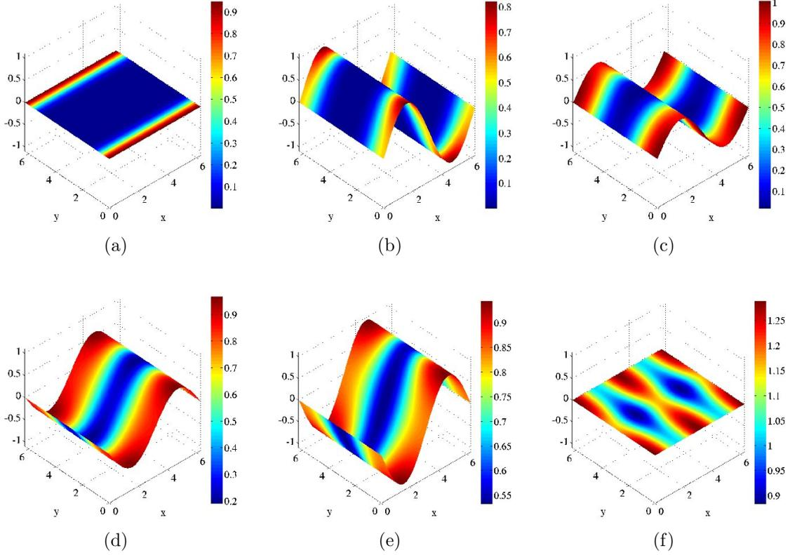
FIG. 6: Front propagation on the substrate at times  $t = 0, \frac{1}{5}T, \frac{2}{5}T, \frac{3}{5}T, \frac{4}{5}T, T$ , where  $T = 2\pi/\omega$  is the period of the pulsation, and  $\omega = \sigma = 10$ . The catalyst is initially centred on  $y = 0$  and initially in the  $y$ -direction until a time-periodic state is reached. In reaching this state, the direction of the variation changes, as evidenced by subfigures (e) and (f).
