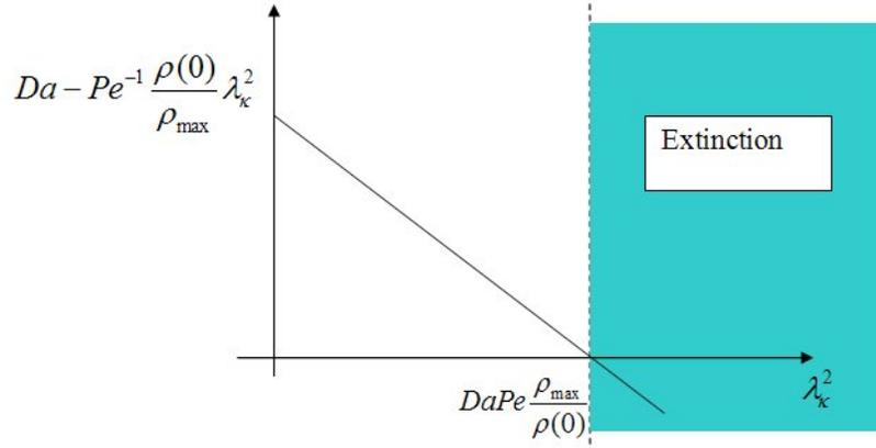
FIG. 2: A schematic diagram showing the possibility for the extinction of the catalyst, when  $\min_{\kappa} \lambda_{\kappa}^2 > Da Pe [\rho_{\max}/\rho(0)]$ . The time-varying scale factor  $\rho_{\max} \geq \rho(0)$  shifts the parameter range of extinction to the right, making extinction less likely. On the other hand, the effective diffusion typically shifts the magnitude of the eigenvalues to larger values, thus moving the system further into, or closer to the domain of extinction.
