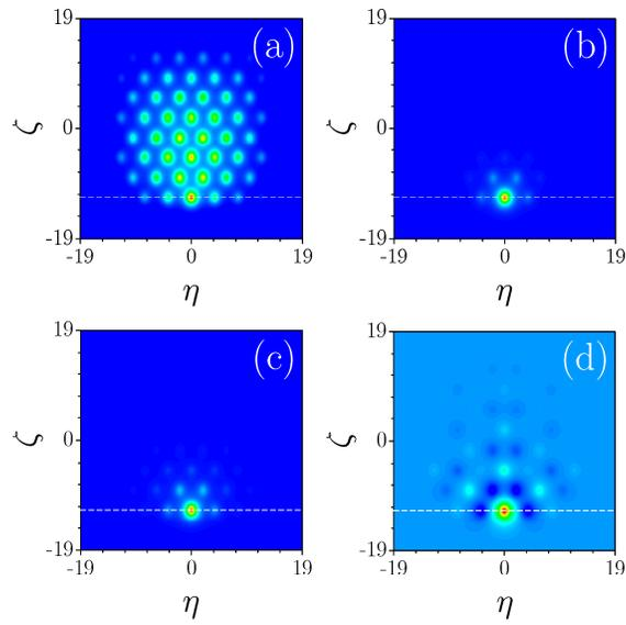
Figure 1. Field distributions for defect surface solitons at (a)  $b = 0.4644$ ,  $p_d = 2.96$ , (b)  $b = 0.512$ ,  $p_d = 2.96$ , (c)  $b = 0.49$ ,  $p_d = 3.1$ , (d)  $b = 0.274$ ,  $p_d = 1.7$ . The white dashed lines indicate the interface position.
