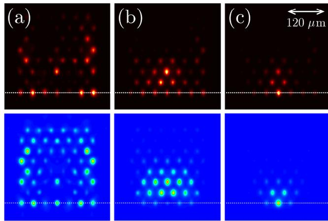
Figure 3. Comparison of the output intensity distributions for an excitation of a surface waveguide in array without defect at  $p_d = p_a = 2.8$ . Top row - experiment, bottom row - theory. The input peak power is (a) 0.18 MW, (b) 1.3 MW, and (c) 3.2 MW.
