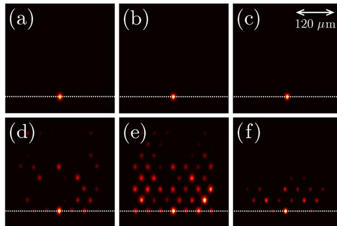
Figure 4. Output intensity distributions for an excitation of (a)-(c) positive surface defect waveguide at  $p_d = 3.03$ ,  $p_a = 2.8$  or (d)-(f) negative surface defect waveguide at  $p_d = 2.7$ ,  $p_a = 2.8$ . Input peak power is (a) 0.2 MW, (b) 1.3 MW, (c) 2.7 MW, (d) 0.2 MW, (e) 1.3 MW, and (f) 3.2 MW.
