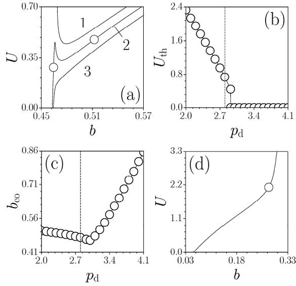
Figure 2. (a) Power versus propagation constant for  $p_d = 2.92$  (curve 1), 2.96 (curve 2), and 3 (curve 3). The circles correspond to solitons in Figs. 1(a) and 1(b). Threshold power (b) and cutoff (c) versus  $p_d$ . Dashed lines indicate the point  $p_d = 2.8$ . (d) Power versus propagation constant for a surface mode existing due to Bragg guiding at  $p_d = 1.7$ . The circle corresponds to profile from Fig. 1(d).
