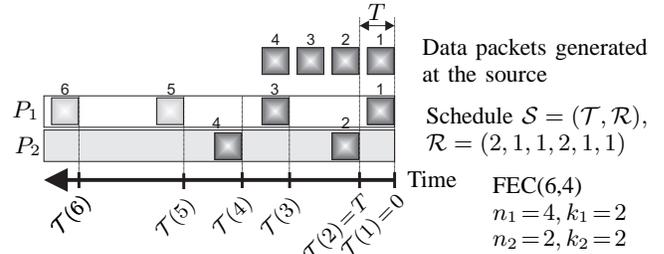
Fig. 4. An illustration of a schedule  $S = (\mathcal{T}, \mathcal{R})$  on  $R = 2$  paths with FEC(6,4). Four data packets numbered 1-4 are generated at the source at equal intervals  $T$ ; the first one specifies time  $t = 0$ . The  $n - k = 2$  redundancy packets are numbered 5 and 6. According to the schedule  $S = (\mathcal{T}, \mathcal{R})$ , the  $i$ th FEC packet is sent at time  $\mathcal{T}(i) \geq 0$  over path  $\mathcal{R}(i)$ .
