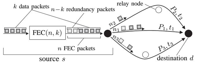
Fig. 1. Illustration of a multipath system with  $R = 3$  paths  $P_1, P_2, P_3$  between source  $s$  and destination  $d$ .  $t_1, t_2, t_3$  are the corresponding path propagation times.  $k$  data packets are complemented with  $n - k$  redundancy packets, and the resulting  $n$  FEC packets are split onto the three paths using the rates  $n_1, n_2$  and  $n_3$ , respectively.
