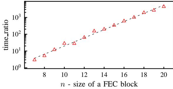
Fig. 5. The time complexity of the effective loss rate  $\pi_B^*$  under an arbitrary schedule (III-A) vs. the even-spaced schedule (III-B):  $\text{time\_ratio}$  is the runtime of Eq. (7) divided by the runtime of Eq. (11). Here we use  $\text{FEC}(n, 0.7n)$  on two identical paths.
