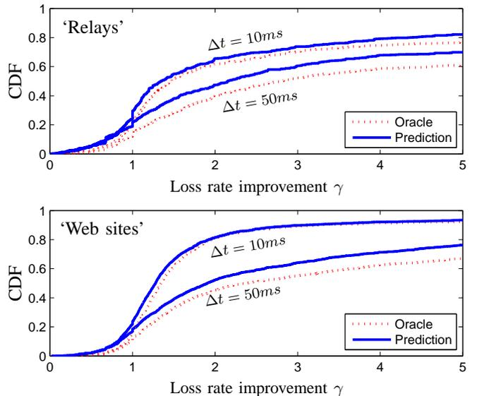
Fig. 10. The effective loss rate improvement  $\gamma$  (by using Spread instead of Immediate) in trace-driven simulations under FEC(10, 8). We use  $R = 2$  independent paths with real-life loss traces; their propagation times differ by  $\Delta t$ . We consider two data sets: ‘Relays’ (top) and ‘Web sites’ (bottom).
