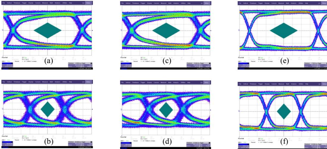
Figure 2: Eye diagrams for signals of (a) 640 and (b) 1,280 Mb/s for a 1.4 m cable with a diameter of 127  $\mu\text{m}$  plus 25  $\mu\text{m}$  of insulation, twisted 2 turns/cm. (c,d) show the corresponding signals for the pixel barrel cable of the same length. (e,f) show the corresponding signals for the pixel barrel cable of 60 cm.
