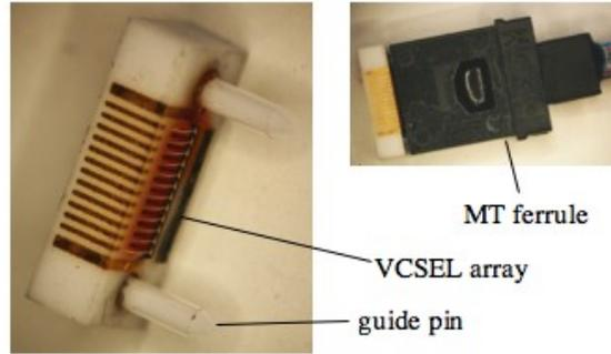
Figure 7: A fabricated opto-pack based on BeO.
