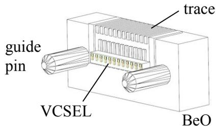
Figure 6: An optical package based on BeO.
