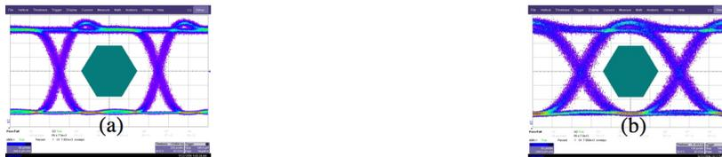
Figure 3: Eye diagrams for optical signals of (a) 1 and (b) 2 Gb/s in a fusion spliced SIMM/GRIN fibre.
