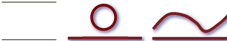
FIG. 3: Progression from Casimir's original configuration of perfect parallel plates, to realistic experimental configurations with different geometries and imperfect surfaces. Here vacuum polarization is probed by the externally imposed boundaries.
